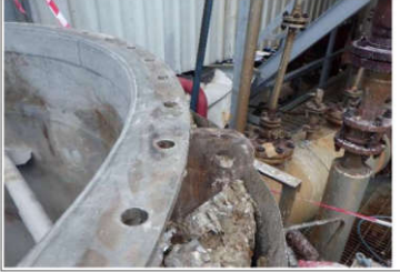
Tag/ part M1-423.Stack Finding Slight corrosion was found on flange.
