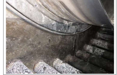
Tag/ part M1-423.Internal Shell Finding Slight corrosion was found on shell
