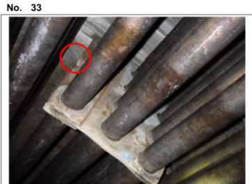
Tag/ part M1-423.baffle plate 14 Zone D Finding Crack on all of the baffle plate weld and corrosion.(Highlight_29)
