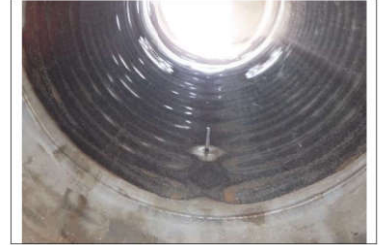
Tag/ part M1-423.Internal Shell Finding Normal Condition
