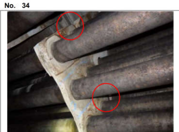
Tag/ part M1-423.baffle plate 13 Zone D Finding Crack on all of the baffle plate weld and corrosion.(Highlight_29)
