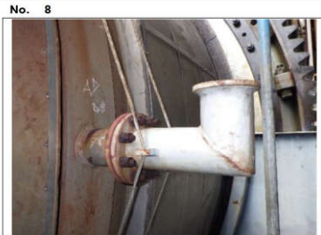
Tag/ part M1-423, Nozzle Finding A minor rust stain was found on the nozzle.
