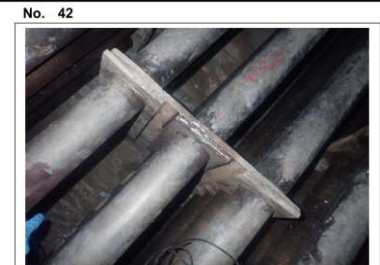
Tag/ part M1-423.baffle plate Zone D Finding Damage Baffle already repaired
