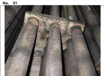
Tag/ part M1-423.baffle plate Zone C Finding Moderate corrosion was found on baffle plate .
