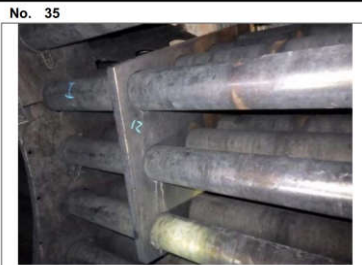
Tag/ part M1-423.baffle plate Zone H Finding Moderate corrosion was found on baffle plate .
