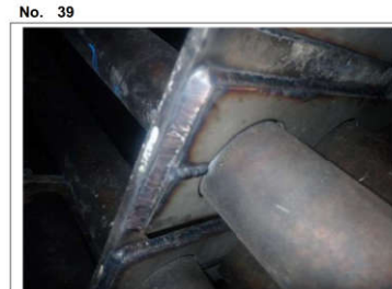
Tag/ part M1-423.baffle plate 14 Zone D Finding Damage Baffle already repaired
