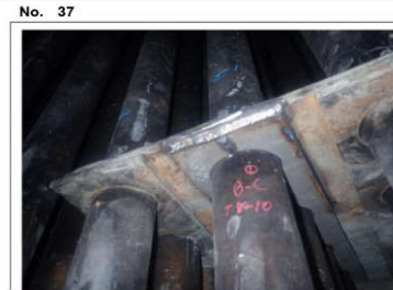
Tag/ part M1-423.baffle plate Zone B-C Finding Damage Baffle already repaired
