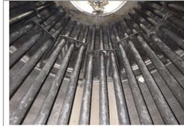
Tag/ part M1-423.Internal Shell Finding Normal Condition
